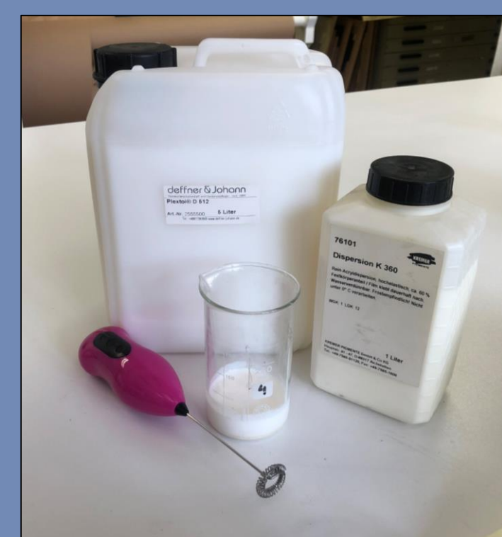
Picture 10 Adhesives Plextol® D 512 and Dispersion K 360 for lining
