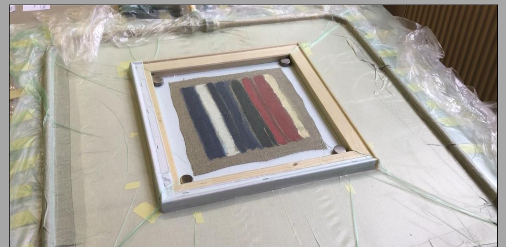
Picture 5 The mock-up inside the low-pressure envelope during lining
