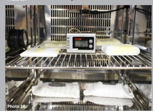
metal staples and duct tape, and the third in Tyvek 1442 fixed with paper tape. Thermohygrometer data loggers (Rotronic HL-1D), with calibrated temperature and relative humidity sensors were packed in the same way as the mock-
