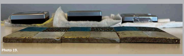
Finally, calibration (ISO/IEC 17025 accredited) of both data loggers and climatic chamber ensures traceability of measurements to SI. The temperature was programmed to change between 21°C and 30°C, and relative humidity between 21% RH and 99%
